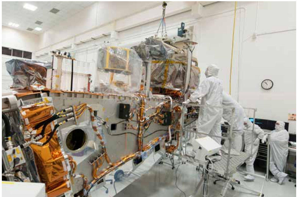
Ball and Raytheon technicians integrate the VIIRS Optical and Electrical Modules onto the JPSS-1 spacecraft in 2015. The spacecraft will be ready for launch later this year. Image Credit: Ball Aerospace & Technologies Corp.
